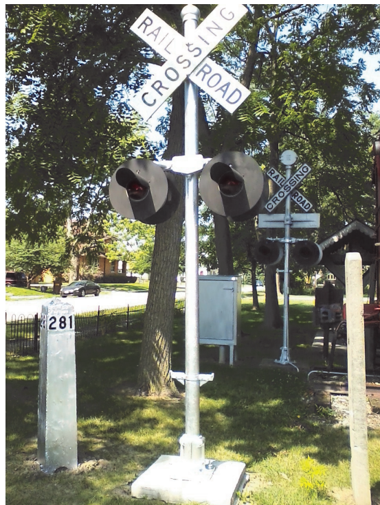
"281" mile marker, a Shannon Street Cincinnati Northern Railroad flasher and a whistle marker. The flasher from Elida, Ohio, installed in the 1990s, and the control box installed in 2002, are in the background.
